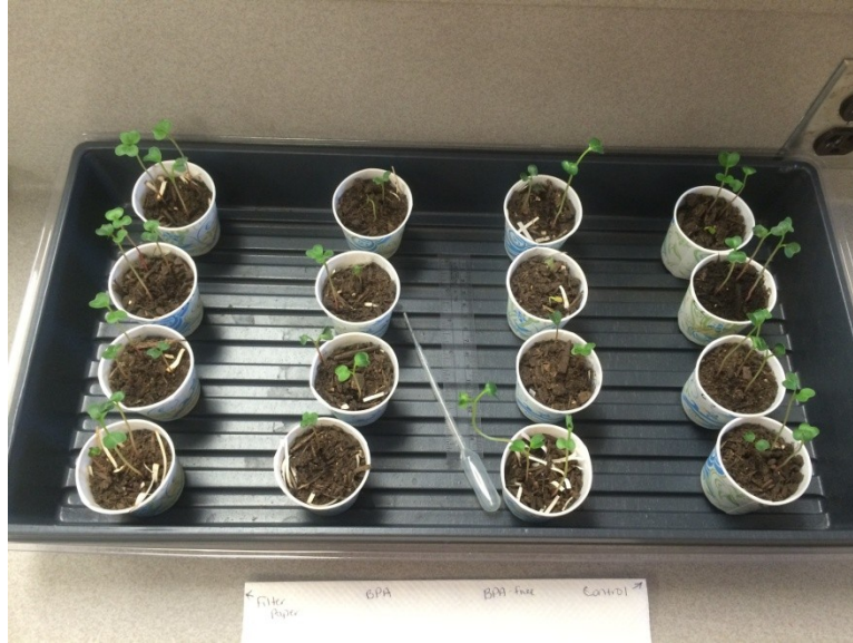
Figure 1. Four groups of radish seeds, one control group and three experimental groups were grown in the lab. From left to right the groups are: Filter paper, BPA thermal receipt paper, BPA-free thermal receipt paper, and control (no paper).
